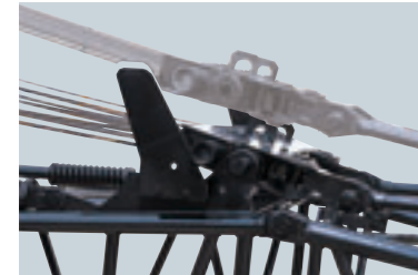
Bridle joint guides adopted for increased ease of boom disassembly and reassembly
